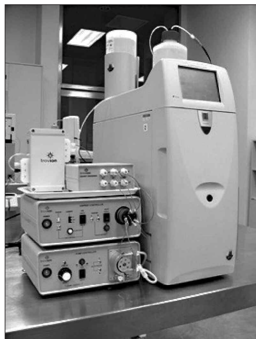
Figure 4: IC system with IonPrep for trace ion analysis.
